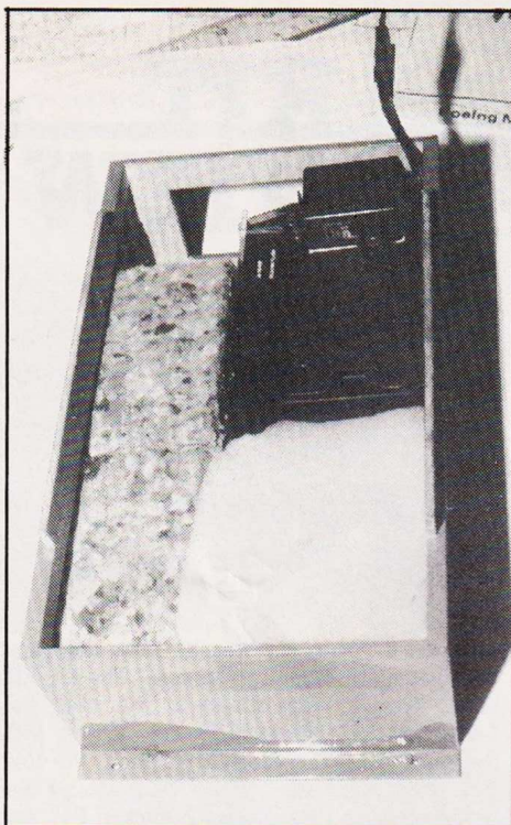
Camera installation as devised by Steve is simple and effective, servo, attached by servo tape, is easily removed for normal use of the camera. Note large dimensions of carrier box.
