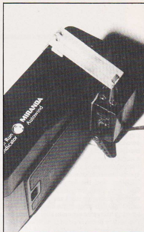
Camera installation as devised by Steve is simple and effective, servo, attached by servo tape, is easily removed for normal use of the camera. Note large dimensions of carrier box.
