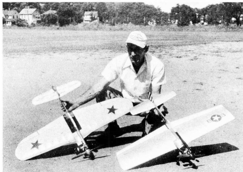
Extra maneuverability is imparted by the use of full-span flaps. For this article K & B 29's were used, but hot 19's ok. Bigger engines get lively.
