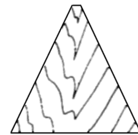
1/16" PLY ACTUATOR BASE. BOLT ACTUATOR TO BASE THEN INSTALL IN THIS SLOT
