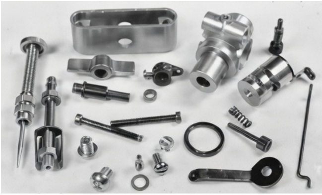
Below: the stripped down throttle assembly.
