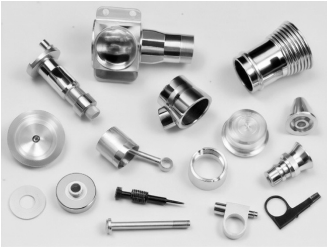
Breakdown photograph showing the components of the Cox Tee Dee .09.
