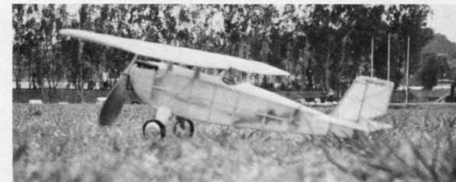
The WP-1 at rest. A single loop of 3/32 rubber about 18 inches long was just right for Walt's model. His model needed 1/32-inch up elevator, and a little washout at each wingtip.
