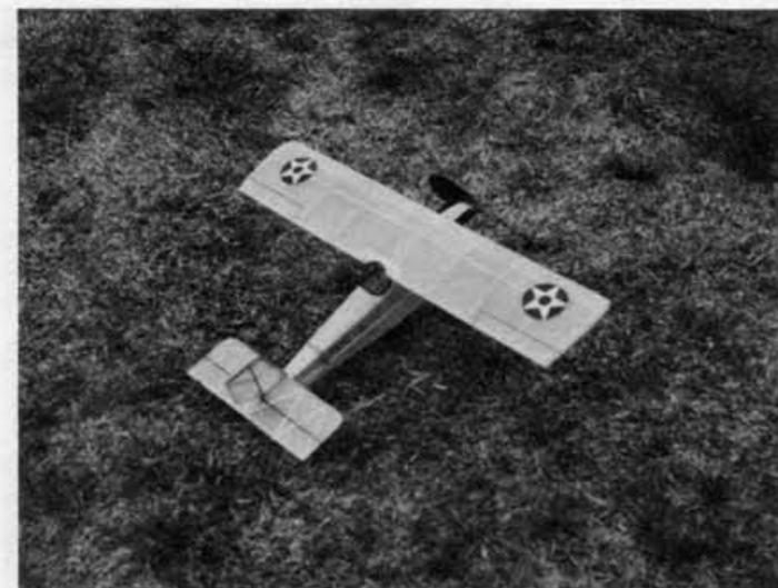
The WP-1 decorated and also seen in skeleton form. An aerodynamically "clean" airplane, it has adequate wing area for a Peanut. Walt's weighed in at 10 grams, and managed 39 seconds in test flights.
