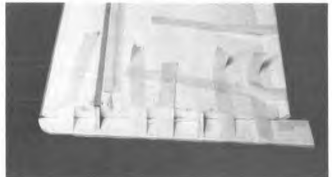
Epoxy and tape both wing tips to core as shown. Note the slot in the wing for the antenna tube and the "Fome Cor ® " gussets.
