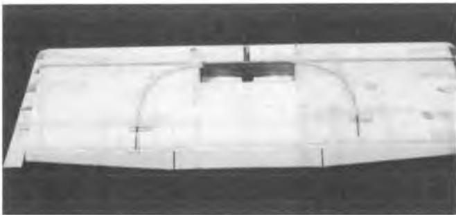
The completed assembly. Do not install the motor mount until covering is completed. Allow to dry overnight, sand smooth with 100, 150, 220 and 400 grit sandpaper prior to covering.
