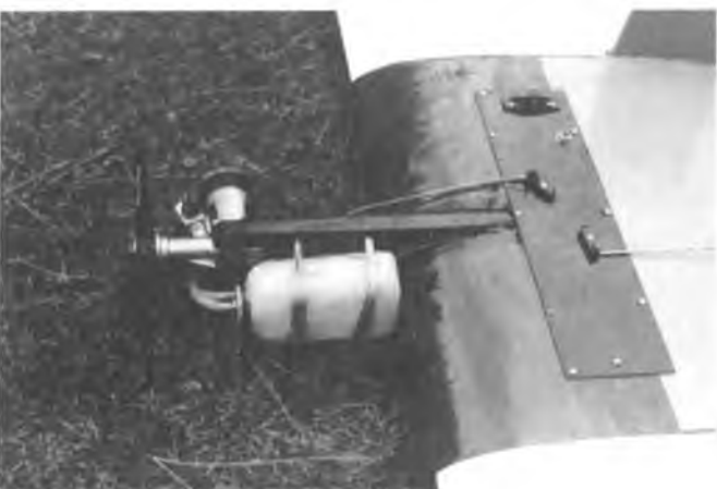
The engine and radio installation in a model using conventional aileron and elevator control.
