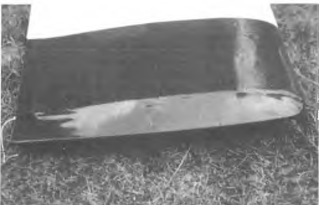
The fabricated wing tip is easily covered with low temperature films.
