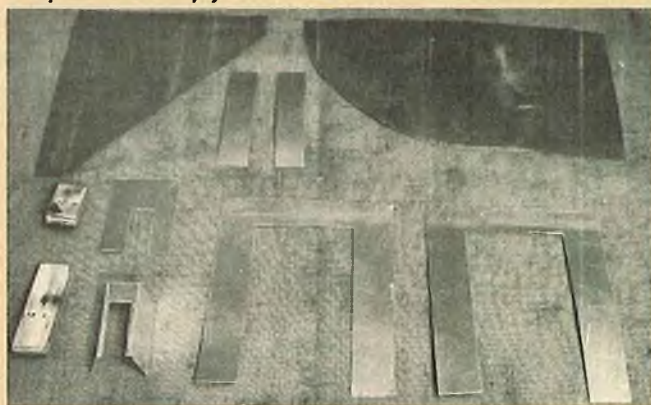
Fixtures and templates used to cut detail into the wing cores. Note the two hot wire slot cutters at the extreme left. Adjacent to these cutters are the templates used to cut the motor mount reinforcement slots. The use of the remaining parts is illustrated in subsequent photos.
