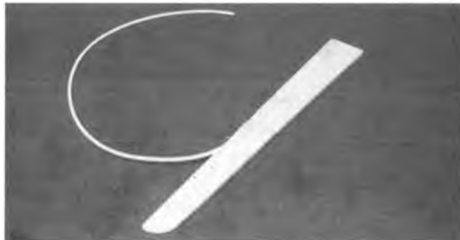
Slot the bottom and inner edge of the right hand wing tip to accommodate the antenna tubing. Epoxy tube in place and use tape to hold till cured.
