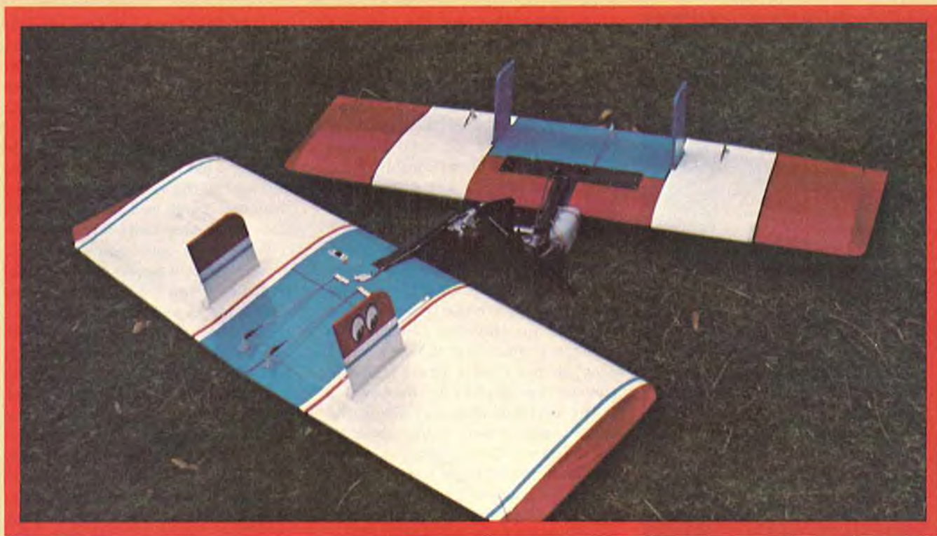
Two versions of the Winger have been built: In the foreground is shown the use of elevons for both pitch and roll control. In the rear is a version using conventional aileron and elevator to control these functions.
