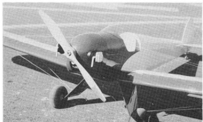
All set to go flyin'. Original model was finished in cream and maroon Monokote, recommended for strength and light weight.
