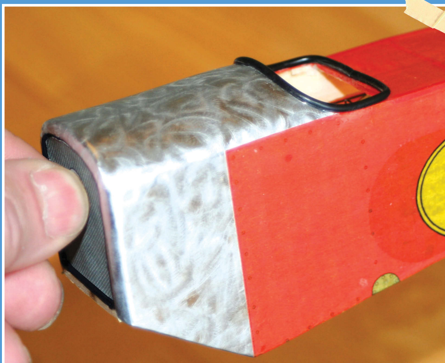
The Oracover ironed onto the nose gives a very good swirled aluminium effect. Cockpit coaming is just insulation stripped from electrical wire.
