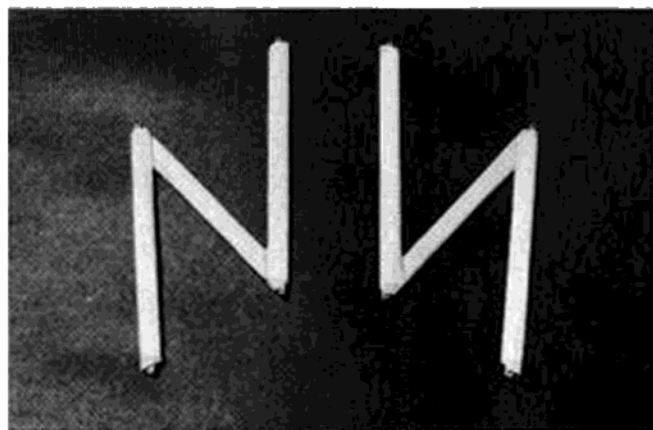
LEFT: "N" struts after being faired with balsa, and shaped. RIGHT: Finished "N" struts bolted to wing attachments. There are numerous ways to accomplish this task; author says feel free to use your favorite method.
