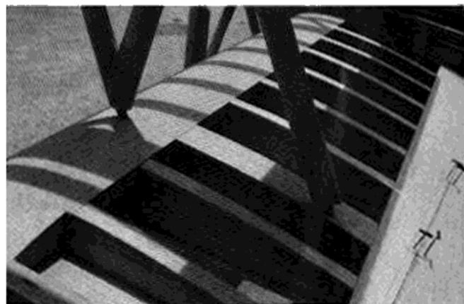
LEFT: "N" struts after being faired with balsa, and shaped. RIGHT: Finished "N" struts bolted to wing attachments. There are numerous ways to accomplish this task; author says feel free to use your favorite method.
