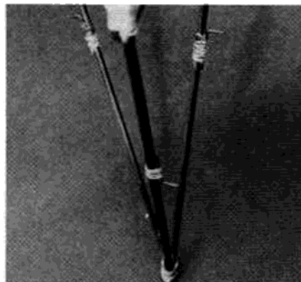
To keep the balsa fairings from turning on the round music wire, wrap and solder small pieces of music wire to struts. Middle piece of balsa "sandwich" is held in place nicely with these.
