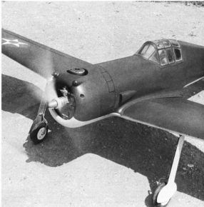
Flaps lowered, nose toward the sky. At right, a ring cowling. Beneath: Full flaps are visible. Photos at bottom show Heath system and muffler recessed into the cowling. Neat and effective.
