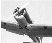
Flaps lowered, nose toward the sky. At right, a ring cowling. Beneath: Full flaps are visible. Photos at bottom show Heath system and muffler recessed into the cowling. Neat and effective.
