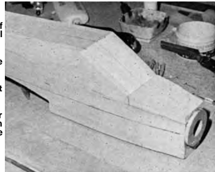
Above: What looks like a canopy is built up of balsa blocks and triangles. Space inside will house battery packs.
