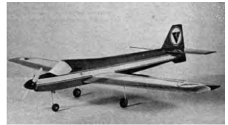
At rest on the gear, Viper has that look of ready action. Note the moveable sub-fin. This is most helpful in wingovers
