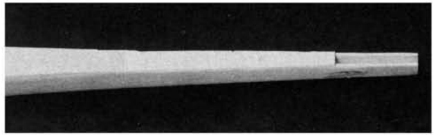
Tail end of fuselage ready for fin to be installed. Last piece is glued to fin then on to fuselage.
