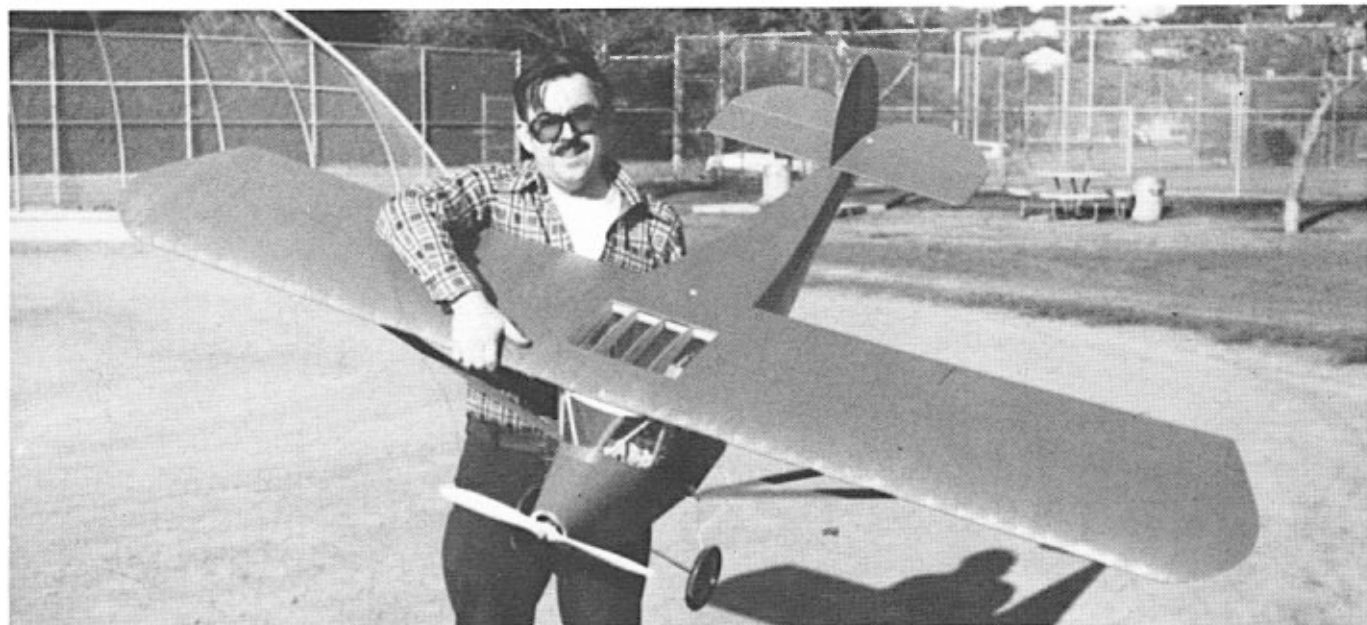
Bob Boucher with his Mammoth Monocoupe, during first flight tests. Design is enlargement of his Astro Flight 50 inch kit for 1/2A glow or .05 electric.
