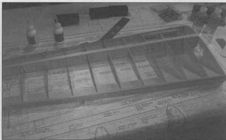
The partially finished right-hand wing panel upside-down on the workbench. Construction is completely conventional D-tube, yielding a strong, stiff, light structure.
