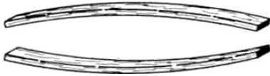
TWO WARPED SPARS INSTALLED THIS WAY WILL RESULT IN A STRAIGHT WING
