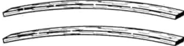
TWO WARPED SPARS INSTALLED THIS WAY WILL RESULT IN A WARPED WING
