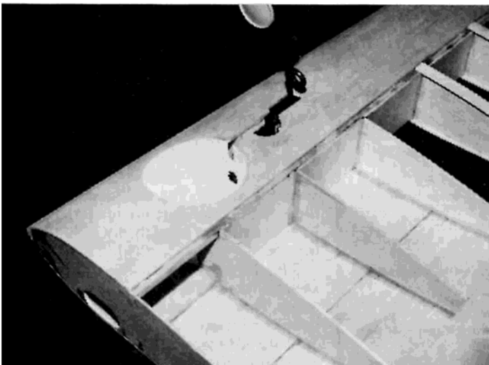
Retract mechanism can be sheeted over or left accessible. Wheel well is cut after gear is installed to insure proper alignment.
