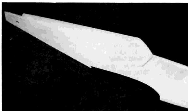
The finished turtledeck. You won't believe how easily you can achieve fiberglass-like shapes with this technique.
