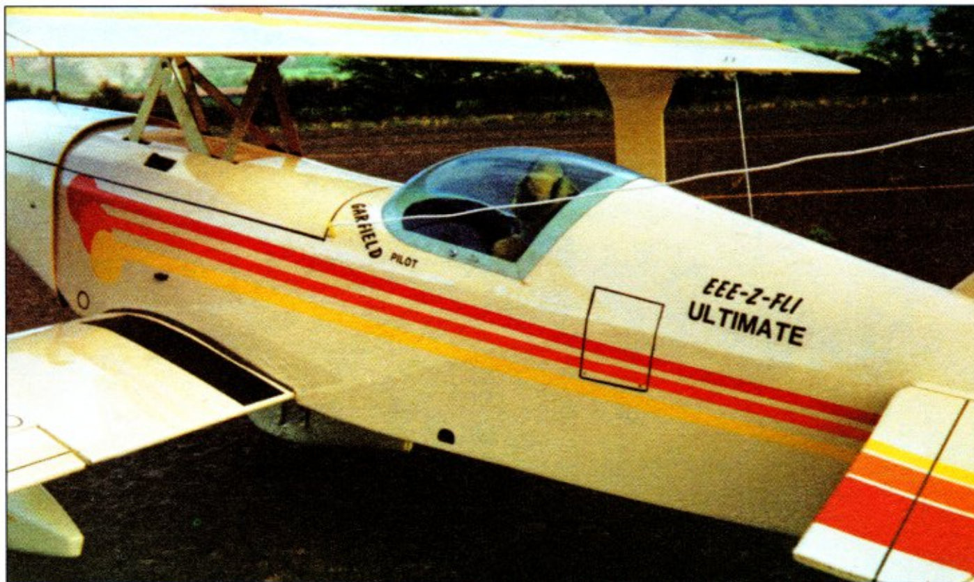
The canopy (in this case, "borrowed" from an EZ Christen Eagle) is secured simply with a couple of small screws. Overall covering is MonoKote, Al's favorite for all of his EEE-Z-FLI projects. Cowl and other small parts are sprayed with Pactra's Formula-U polyurethane.
