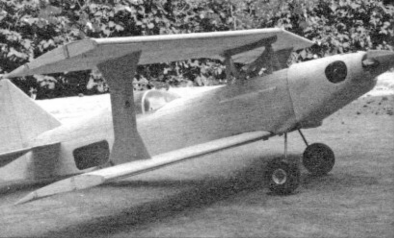
Ready for covering and paint, this view shows off the Ultimate's straight lines and simple construction. Note also the experimental short landing gear, which probably improves the ground handling a bit but doesn't look as good as the longer gear.
