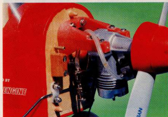
Plumbed in and ready for engine trials. Remote needle is a sensible safety precaution and helps keep a clean profile.
