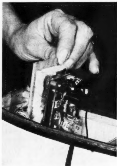
Twin hard-tube receiver mounts on foam rubber. Use Pliobond to attach foam to tray, receiver.
