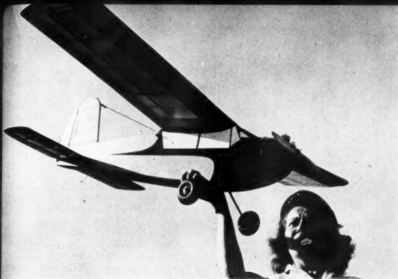
Following popular practice, Triple Threat is easily built. A 15% thick wing, square cross-section prevent excessive dive speeds which interfere with outside loops. But climbs well.
