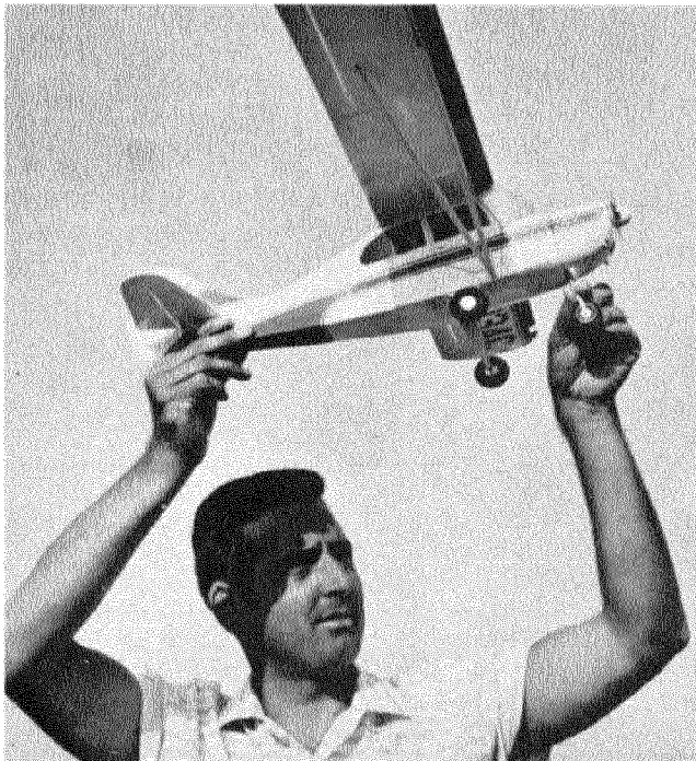
Scale tail surfaces and near-scale dihedral make Lutz's Champion exceptionally accurate free-flight scale. Yep, the door works!
