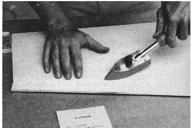
Pin elevon in place on wing and iron X-hinge down on both sides.
