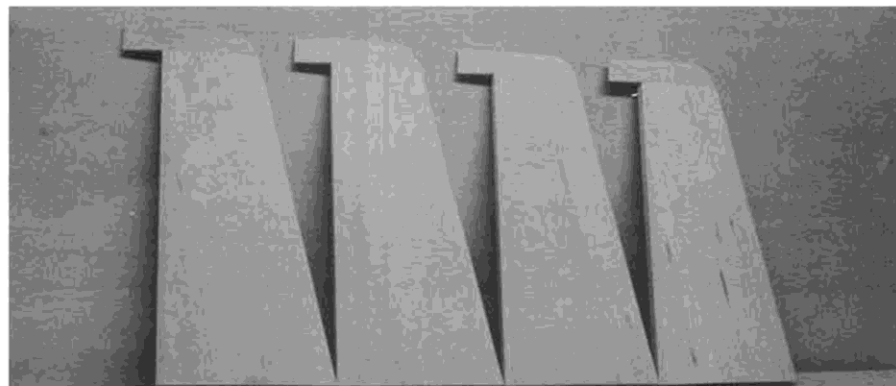
Four stabilizer halves, ready for joining. (The author builds these airplanes almost on a production line basis, which is why there are so many stabs.)
