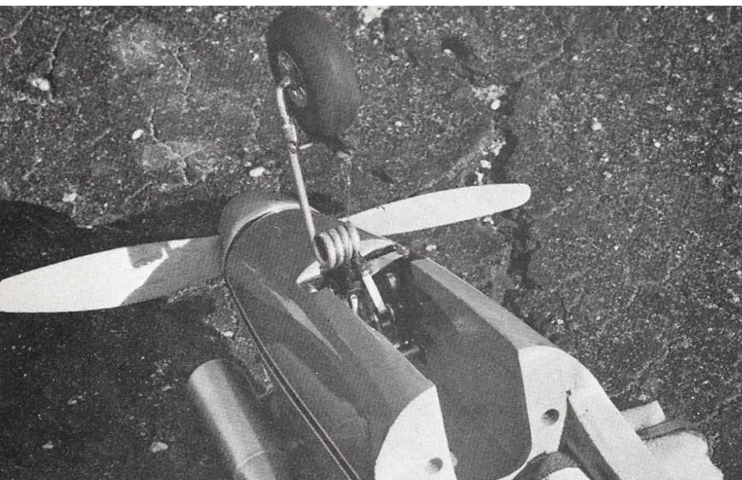
Close-up of the ProLine nose wheel installation. ProLine retract gear is a Chidgey design.
