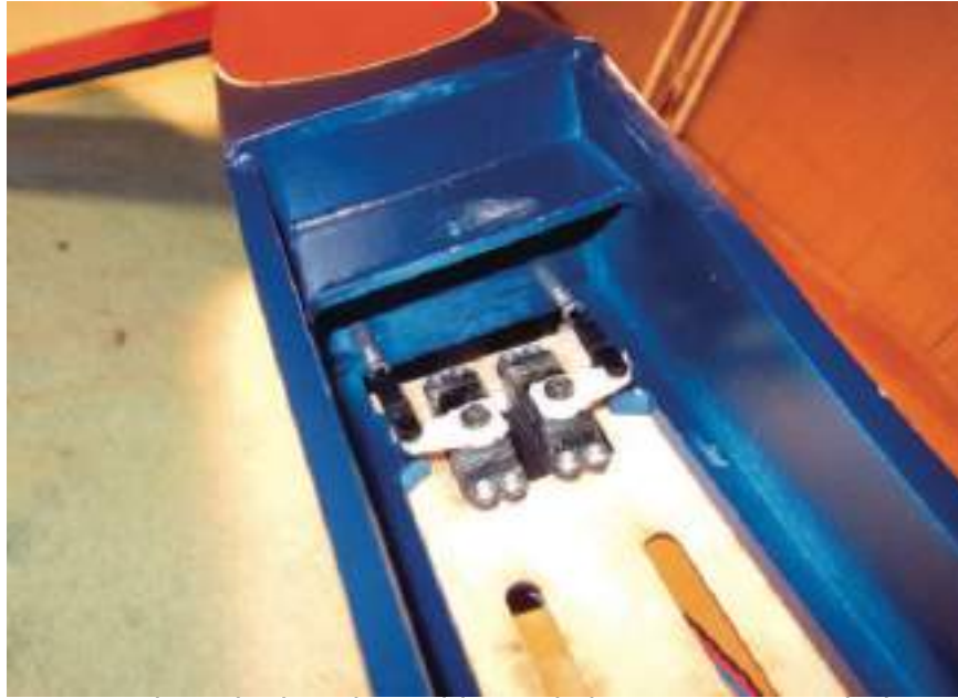
Here's a closer look at the rudder and elevator servos with the push-pull rods and DuBro links installed.
