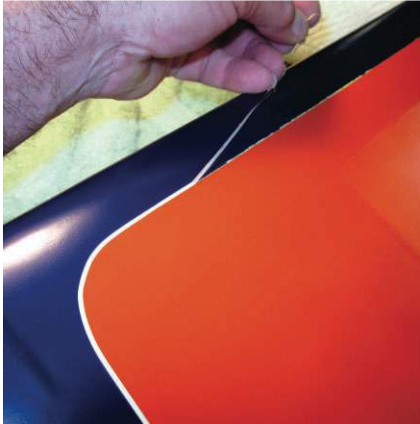
On the bottom of the wing, the fine line tape wasn't as anxious to let go, so I'm pulling it off separately.
