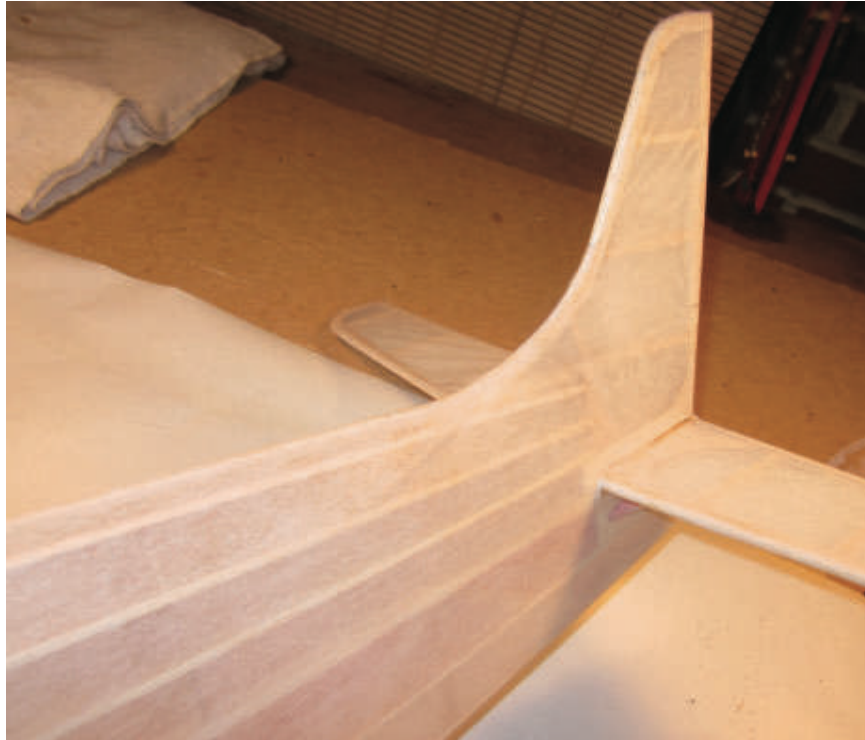
Here it is again from the other side, with the first coat of clear nitrate dope applied.
