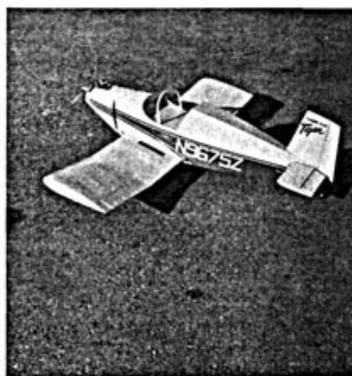
Poly-hedraled wings with eight degrees on each side, add turn stability.
