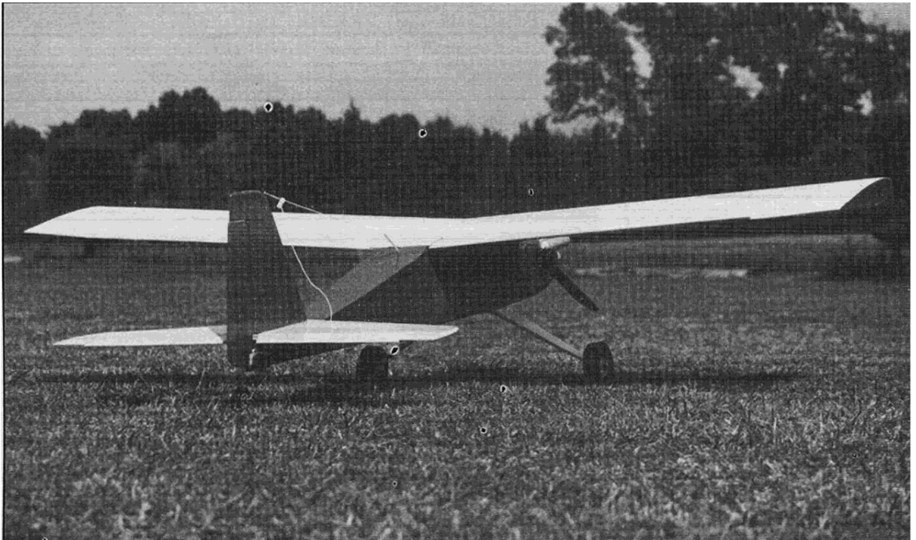
Generous tail feathers contribute to rock-steady trainer stability in a very agile aircraft. Moderate dihedral in this configuration does not detract from formal aerobatics.
