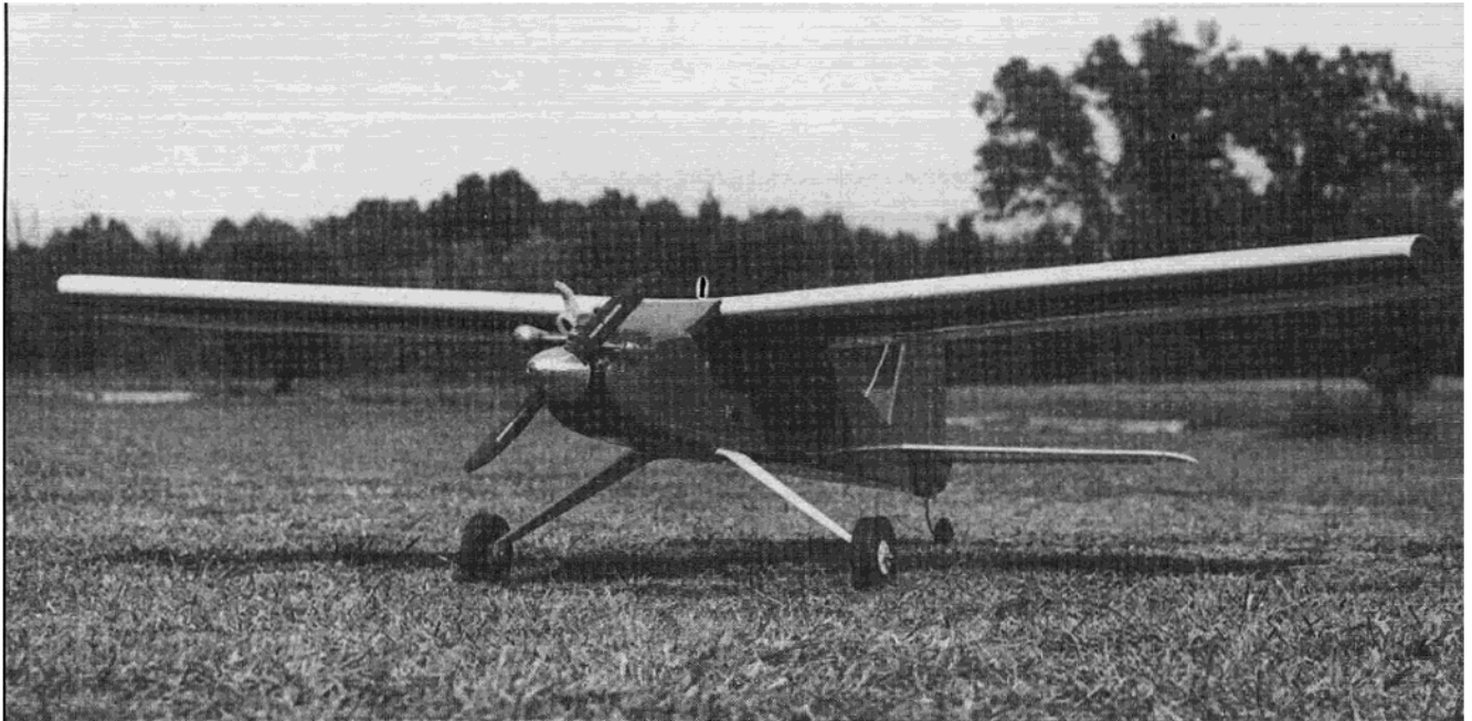
Tern sits at an ideal angle for easy take-off and landings. The 15% thick symmetric airfoil is from the NACA series used on the B-17. Prop is 10 x 5 antique Master Airscrew.
