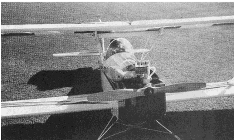
Prototype had an O.S. 108 2-stroke in front and had super performance.
