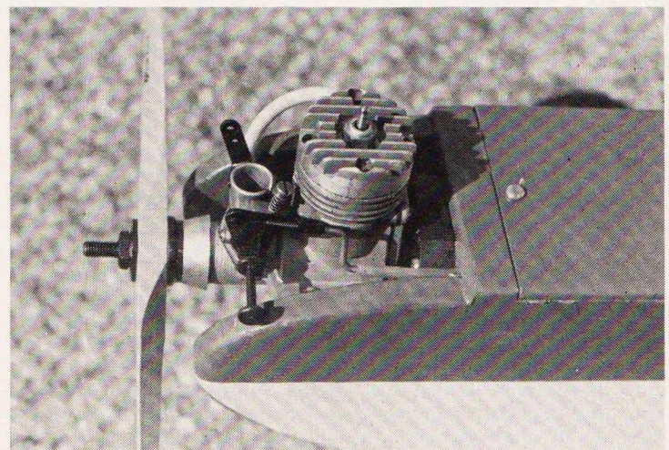
The photo above shows the underside of the tail and the control pushrods. The horns that are provided have plenty of adjusting holes. The Fox .15 installed ( below ). Throttle arm points up. The linkage on left, the engine is very accessible for tuning and clearing.
