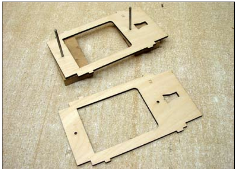
ABOVE: F2 is being assembled on the registration pins, thick CA is used to laminate the two parts.
