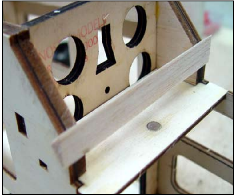
ABOVE: 3/8" Triangle stock installed.
