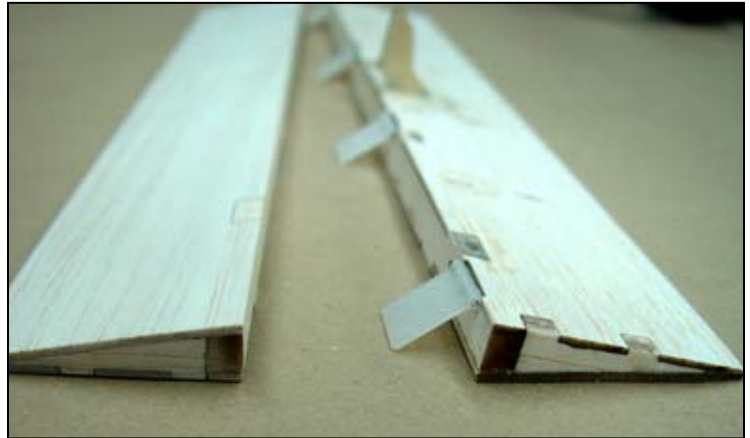
ABOVE: The assembled flaps, on the right with the control horn and the hinges temporarily installed. These will be removed and the final installation will be after the flaps are covered.
