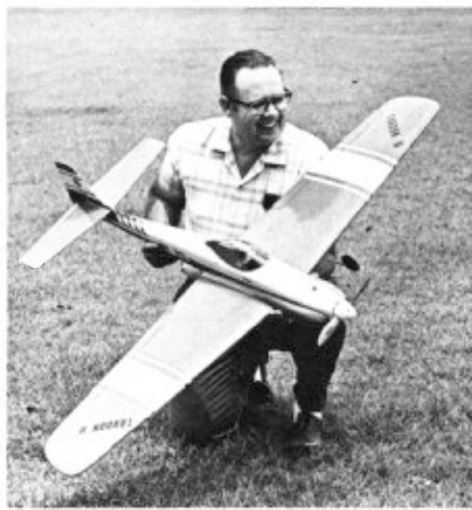
Jack Sabine displays the fairly long high-aspect ratio wing which gives Tardon its fantastically quick pylon turns.
