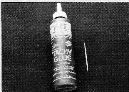
■ LEFT: This technique involves putting lines of glue across the ribs to simulate the rib stitching cord. The glue to use is called Aleene's Tacky Glue, available at craft stores. It's a white glue that dries clear and doesn't get hard. RC-56 might work also. ■ CENTER: Use a soft pencil to lightly mark the stitch locations. If you have a full-scale model to copy, space the stitches accordingly. The author used a 1/2-inch spacing on his sport scale Skybolt. ■ RIGHT: Put a blob of glue on a piece of wax paper, pick up some glue on a toothpick and make a short line with the glue on each mark. Let them dry thoroughly.
