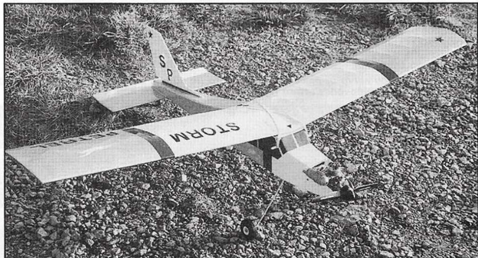
An old, but reliable, OS Max 20 was used in the prototype. Larger engines are not necessary due to lightweight construction.
