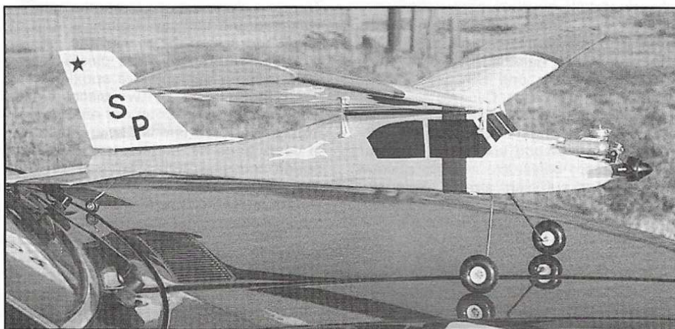
Assuming a classic taildragger pose; the design incorporates good ground clearance to minimise prop strikes.
