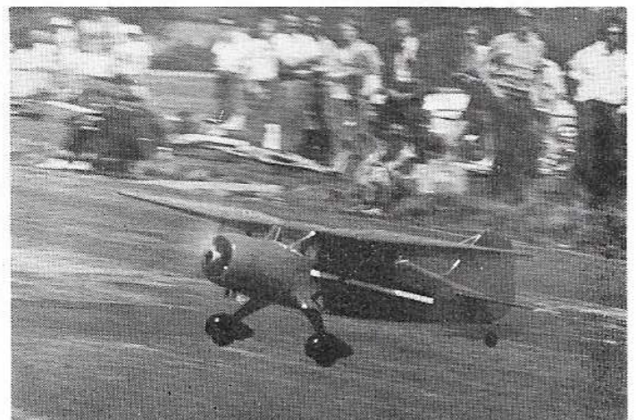
This "starting" snap shows well the Lysander -like wing-thickness double taper—the Reliant is sometimes referred to as "Gullwing" due to this appearance. Below: up . . . and away!
