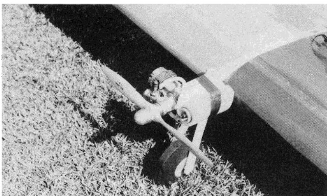
LEFT: Rear quarter view showing completed tail assembly. Also 1/16" M.W. pushrods and plastic guides taped to boom. RIGHT: Front quarter view showing tank taped to pod with foam rubber cushion.
