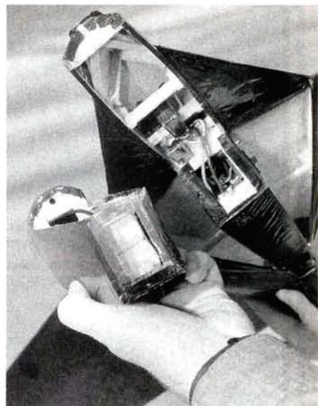
The battery compartment/nose has been removed. A small dowel is inserted into a hole in the back face of the removable nose, and a small Carl Goldberg* hatch lock locks the rearmost piece of the battery compartment to the fuselage with a sideways movement of the compartment. A hard landing will dislodge the battery compartment without damaging the plane.
