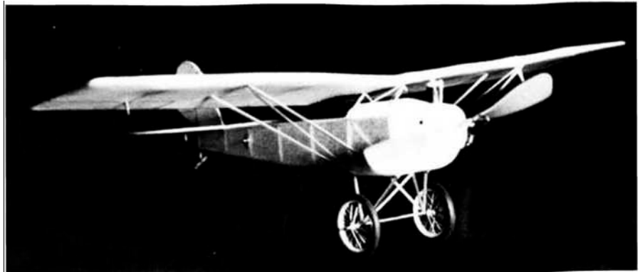
Check the little Stahlwerk against the three-views and you'll see that Walt made very few alterations to the scale outline. The narrow landing gear tread has no effect on ROG's.
