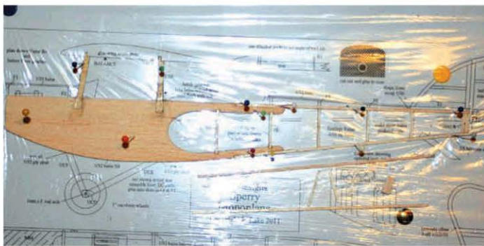
Totally conventional, the fuselage sides are built over the plan in the usual way.
