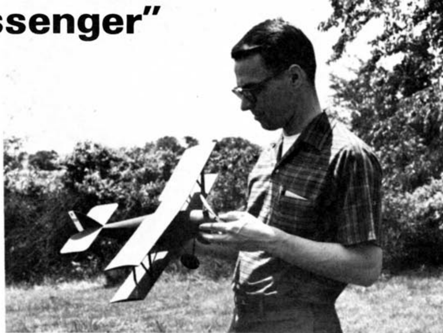
John and his Sperry "Messenger." Wing surfaces are of sheet, saves time for paint detailing. Keep it light, balance and trim the ship with care.
