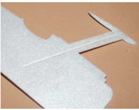
I used a steel rule to make a groove for the carbon rod stiffener to fit into before gluing it in place.
