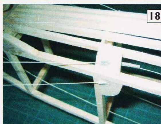
18: Detail of the rear fuselage showing how control runs for a scale-like closed loop link to the servos should be fitted.
