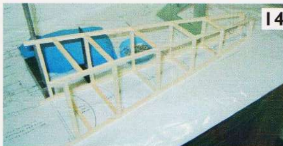
14: The basic box structure of the rear fuselage, built from 1/4" square balsa.
