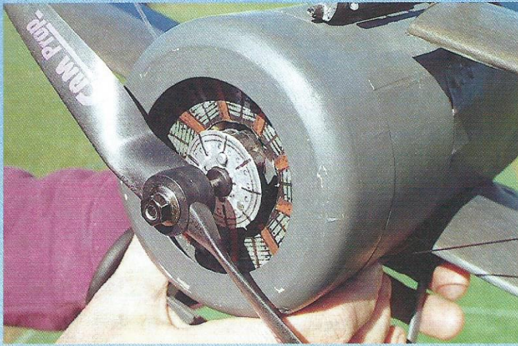
A spot of engine detail is essential inside that prominent cowling ring. Speed 400 motor is carried on laminated 2mm liteply mount for added strength.
