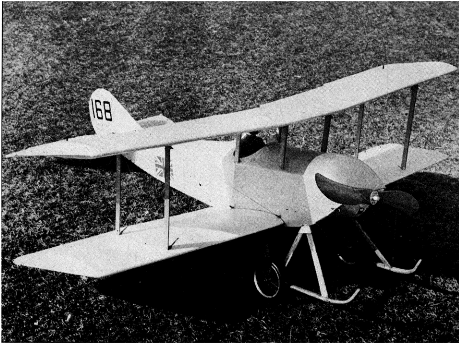
The Tabloid is covered with Super Coverite and painted cream, except for the aluminum areas around the nose.
