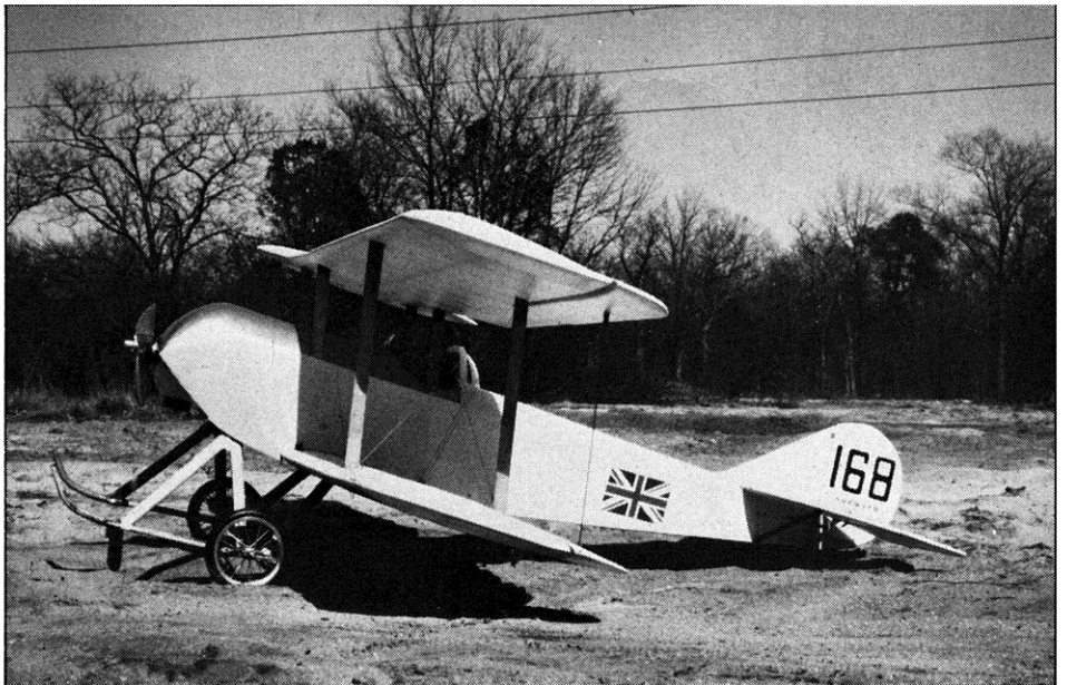
The nifty nose skid adds a nice touch to the author's model, but don't expect it to prevent too many noseovers.
