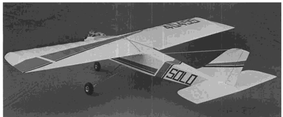
Three-quarter rear view accents wide landing gear tread. Lack of surface spars permits smooth airfoil along full span of wing. Sheet tail surfaces add to ease of construction.
