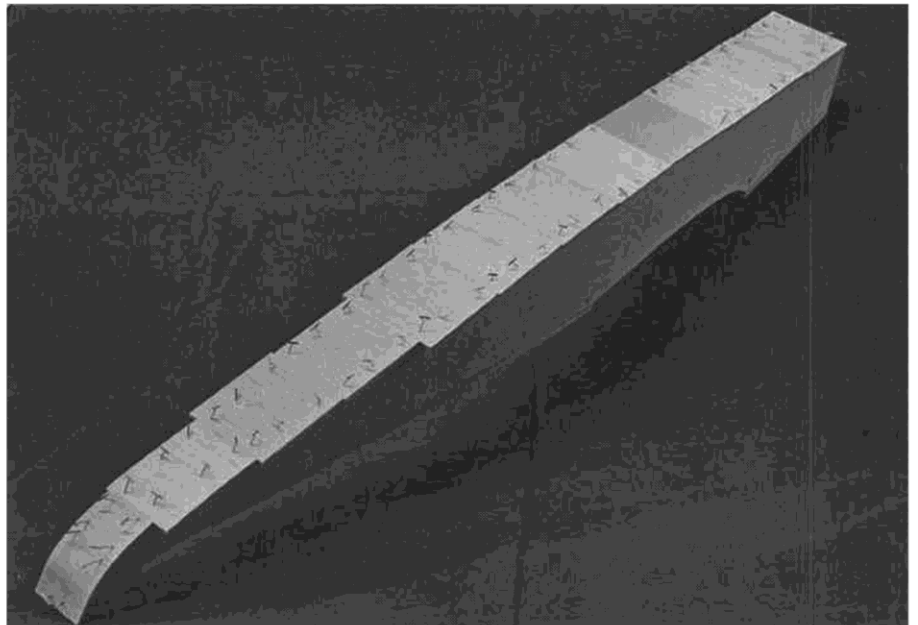
Completed bottom planking, ready for drying. When dry, carefully trim off excess with a razor blade or Uber Skiver, and sand to a smooth finish.
