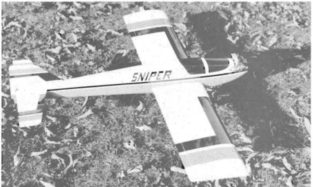
Cover the airplane, reinstall the engine, tank, and radio equipment. Check the balance and surface area throws. Go out and fly it.
