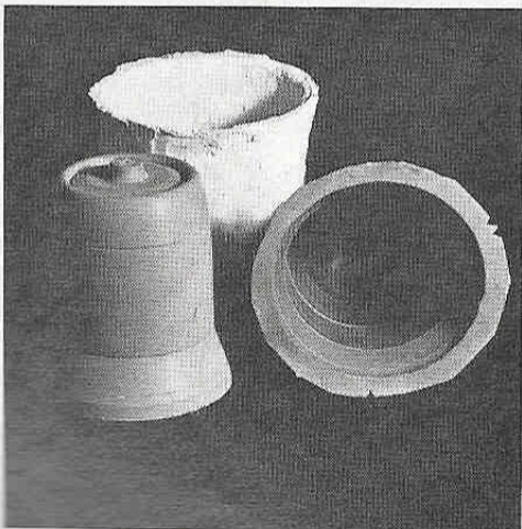
Photo below: The male plug for the cowling was turned on a lathe. Latex mold at right created from the male mold and the "plaster pot" supports the latex mold when laying up fiberglass.
