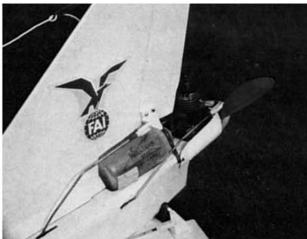
Aft section of Skycar showing Max .10, fuel tank and rudder, elevator, and throttle linkages.
