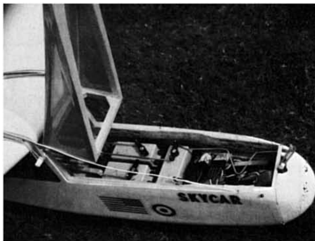
Radio installation in forward section of model. Note "V" bend in nosegear linkage to protect servo.
