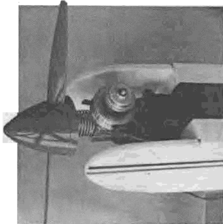
Cox .049 Dragonfly engine with throttle control and 20cc clunk tank. Effective throttle from idle to full power. Power of the Dragonfly is less than a TD, but can be improved with a TD glow head. Still plenty of power to fly the Simple CAP.
