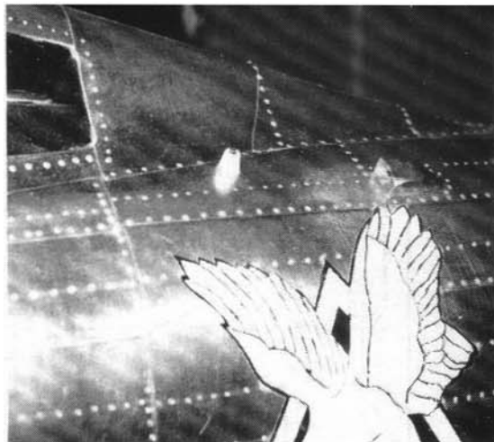
The antenna insulator and scoop are shown.
