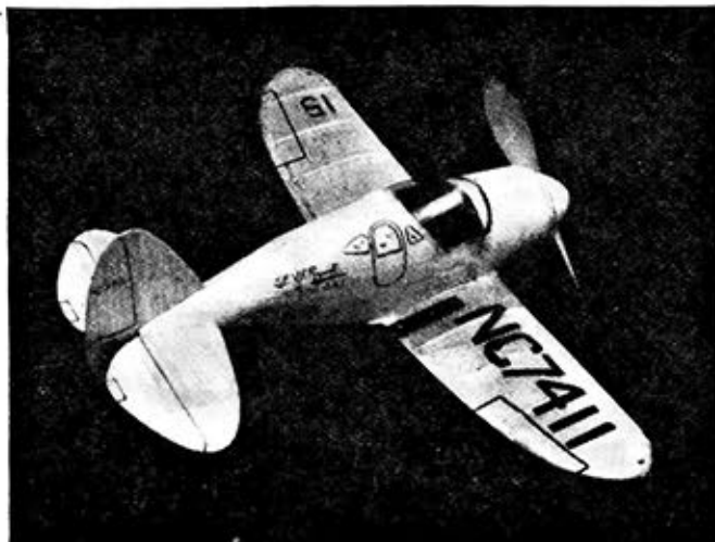
The large tail surfaces give stability
